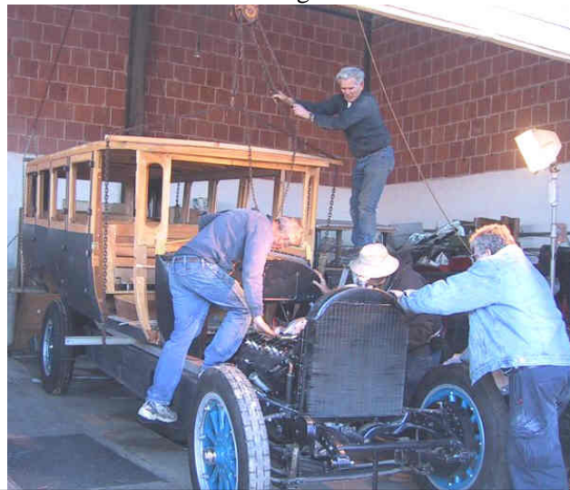
Frank Ball (top), Carl Calvert (left), Sherman George (right) and Ed Carry (center) line up the stage body with the 1924 Cadillac chassis
