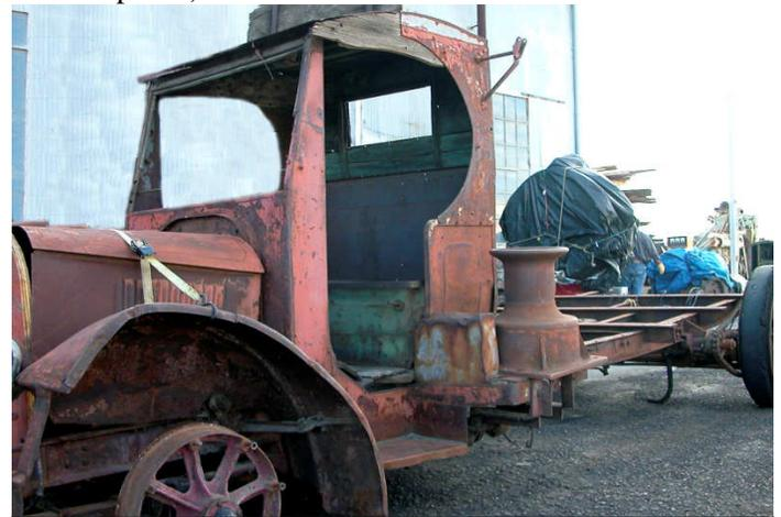
1919 Fageol low-bed truck. Note the power-take-off driven capstan to the left of the cab
