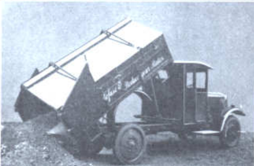
All-metal closed roof refuse body designed by Bean Cars, Ltd., England. The roof consists of four spring loaded covers which, when released, raise automatically.
