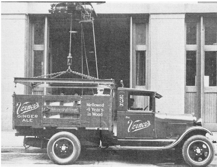
*The body is removed and replaced using an electric hoist. The body is lifted onto a low dolly upon which it can be pushed to the unloading station, then to the loading station and then returned to the truck.*
