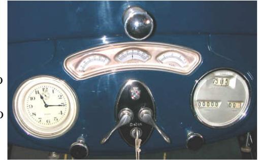
*This instrument group mounted on the dashboard of the Stage. The clock is on the left, the speedometer on the right and the oil pressure, amperes and fuel pressure gauges in the top center. The ignition switch, headlight switch and ignition key are located in the bottom center.*
